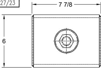
SEISMIC VERTICAL LIMIT-STOP, 1 DIA. MAX. STANDARD NUTS AND WASHERS, TIGHTEN TOGETHER (SEE NOTES 1 & 3)
